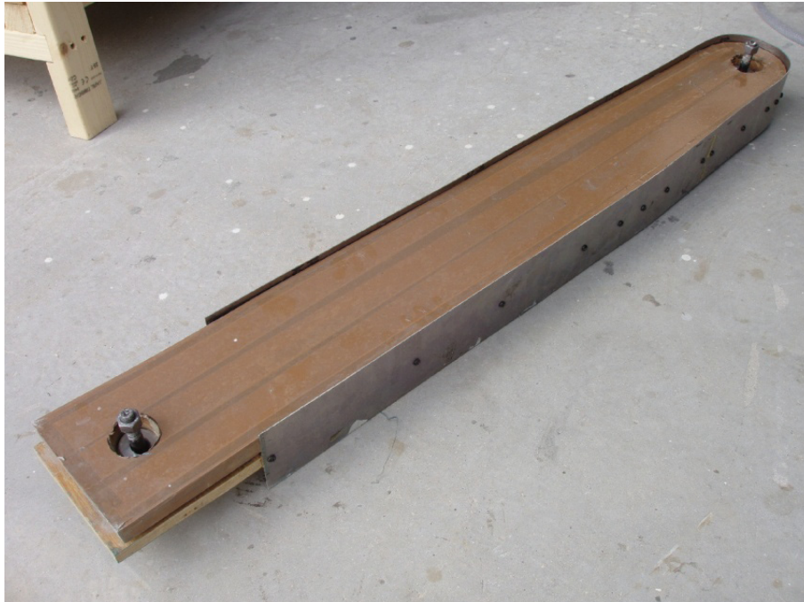
Fig 3: Spar Boom Mould Assembly
