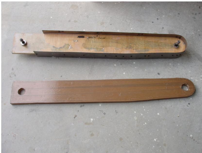
Fig 2: Spar Boom Mould Tool and Timber Intensifier Board
