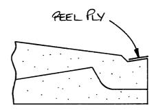
Fig 3. Flap core trailing edge detail.
