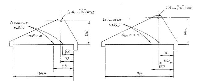
Fig 8. Flap plate positioning jigs (dims in mm).
