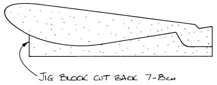
Fig 2. Flap core in jig block.
