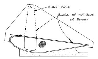
Fig 12. Flap hinge plate temporarily attached to jig.
