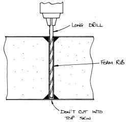
Fig 10. Section through flap at rib area.
