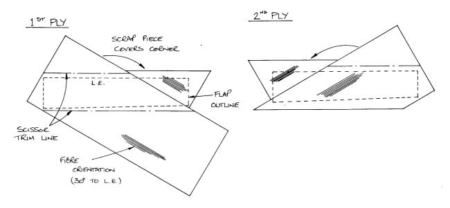
Fig 4. Positioning 'uni' cloth for skin lay-up.
