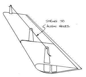
Fig 14. Aligning FL2 hinge plate with FL1 and FL3.
