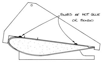
Fig 11. Jig temporarily attached to flap.
