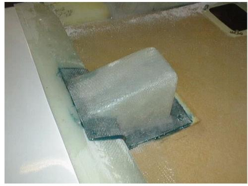
Fig 28. Aileron mass balance box bonded into place.
