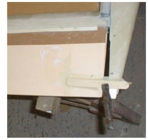
Fig 29. Aileron clamped in neutral.
