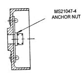
Insert the end cap with the anchor nut attached into the end of CS10 with rapid epoxy between the mating surfaces. The two end caps must be as square as possible to each other to minimise misalignment of the pivot bolts. Any remaining misalignment will be accommodated for by the self-aligning bearings that will be mounted to the support brackets. The rapid epoxy is used as a liquid shim only in this application.
