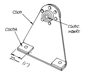
Fig 5. CS09A cuddle plates bonded to CS09 bracket.
