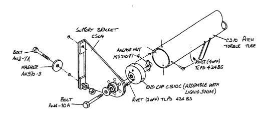
Fig 3. End cap installed in torque tube.
