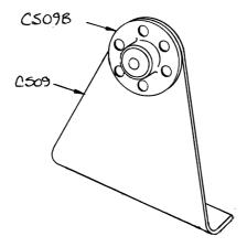
Fig 4. CS09 bracket with CS09B bellcrank assembly.
