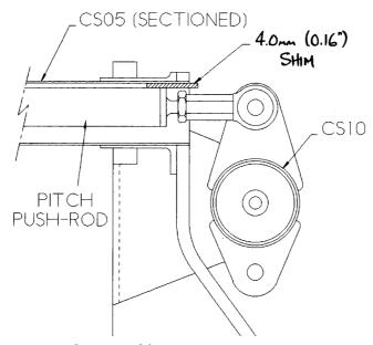
*Fig 7. Pitch push-rod to cross-tube assembly.*
