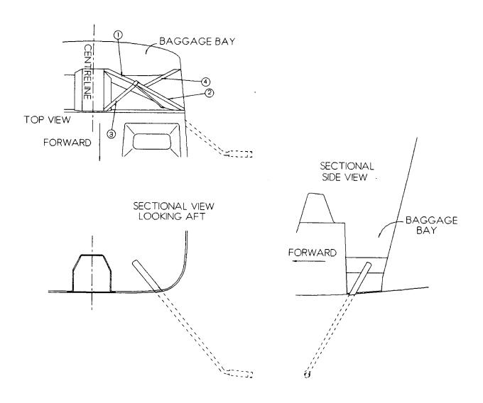
Fig 4. Detail of socket tube and rib installation.
