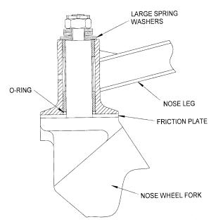
Fig 6. Arrangement of nose-gear housing and fork assembly.
