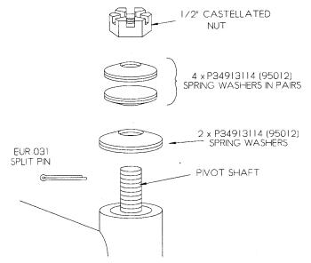
Fig 7. Arrangement of spring washers.
