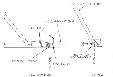
Note: FS70 is 2.25" aft of the forward face of the port spar, and 1" aft of the forward face of the starboard spar.
