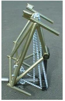
Fig 9. Routing of cable - shown external to aircraft for clarity.
