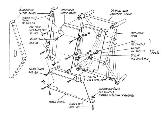
Fig 1. Exploded view of firewall assembly (monowheel frame shown - trigear is similar).
