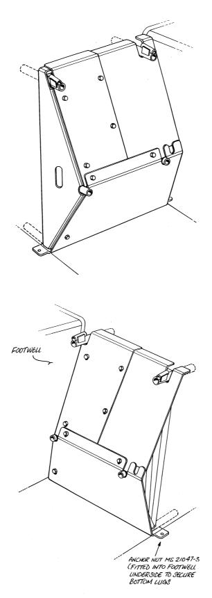
Fig 2. Firewall panels installed positions.
