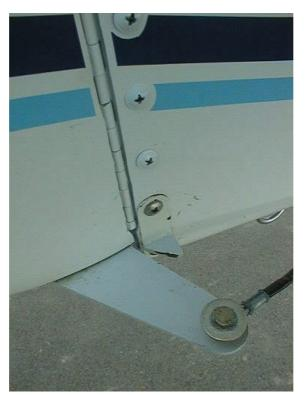
Fig 10. Photo of starboard rudder stop.
