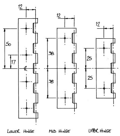
fin with a cleco in each Fig 3. Rudder hinge bolt attachment hole locations. hinge.
