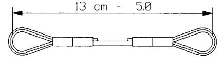
Fig 8. Tailwheel drive cable.
