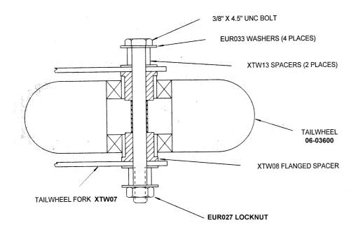
Fig 6. Section through tailwheel axle.
