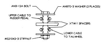
Fig 9. Detail of starboard cable fixing.
