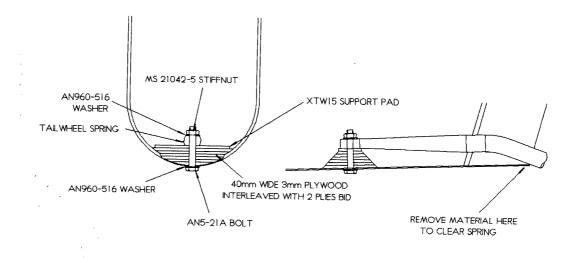
Fig 4. Forward mounting of tailwheel spring.
