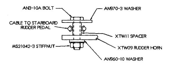
Fig 5. Starboard rudder cable termination at rudder.
