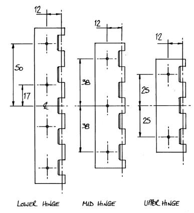
Fig 3. Rudder hinge bolt attachment hole locations.
