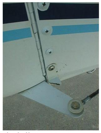
Fig 5. Photo of starboard rudder stop.
