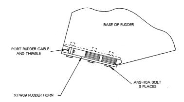
*Fig 4. Port rudder cable termination at rudder.*
