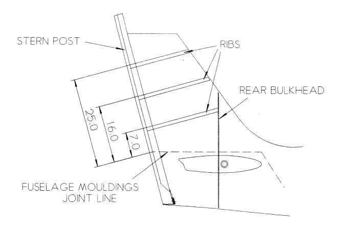
Fig 1. Position of ribs in fin.
