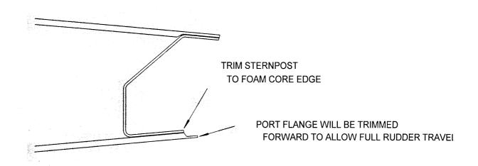
Fig 2. Section through fin trailing edge.
