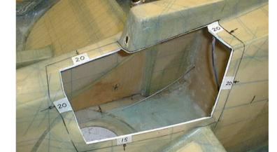
Fig 4. Tunnel after cutting.
