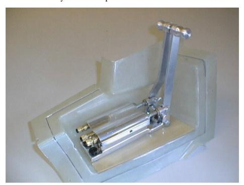
Fig 7. Platform / master cylinder sub-assembly.
