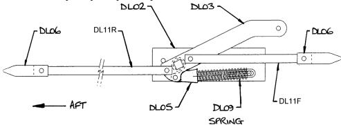
Fig 1. General arrangement of door latch components.
