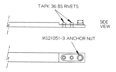
Fig 3. Attachment of anchor nut to push rod.
