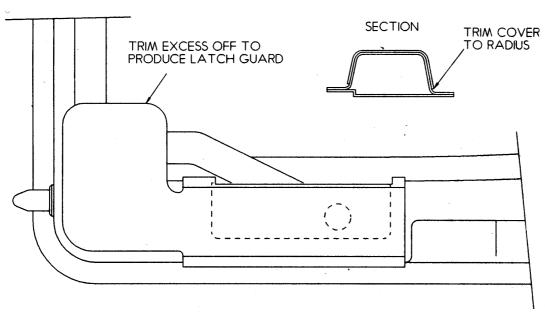
Fig 9. Latch mechanism cover plate.
