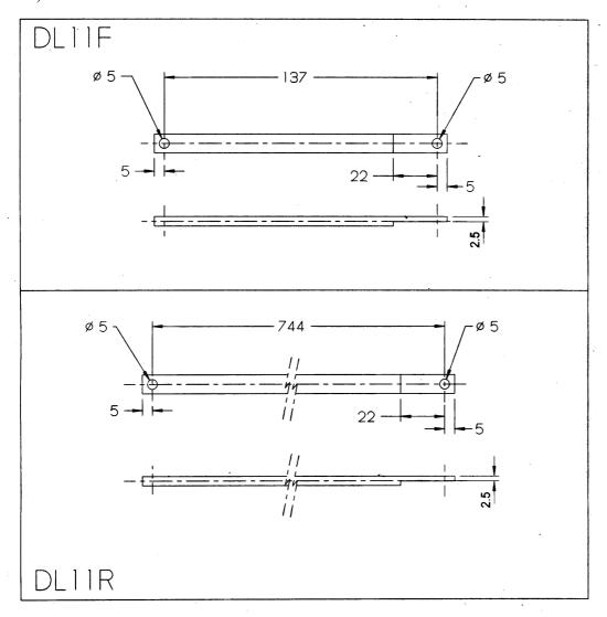
Fig 2. Fore and aft push-rods.
