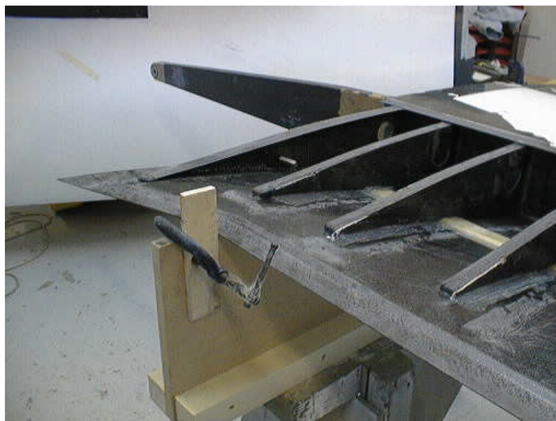
Fig 20. Clamp fitted to stop wing shifting aft.
