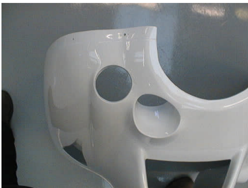
Figure 3. Lower cowl showing completed extra inlet.
