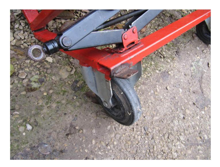
The (slightly rusty) tabs above the wheel on each side are screwed to laterally folding fixing points in the covered trolley with wing nut bolts. The wheels run in U shaped channels in the trailer. Together with a system to secure the tail wheel spring, this allows secure trailing of the fuselage with no other fixing
