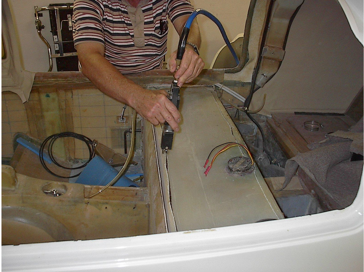
Figure 5 Cutting the top out of the tank.
