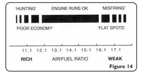
An engine will run, indeed run quite well, at mixtures that are richer or weaker than those specified by the motor manufacturer. However, at settings richer than the manufacturer recommends, there is a loss in economy, and at very rich settings, typically 8% to 10% CO, the onset of poor running occurs, characterized by the particular engine sound that is known as "hunting".
