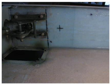
Fig 1. Marking hole position on spar.
