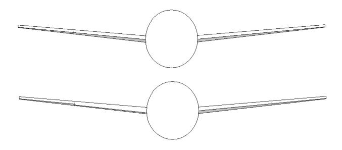
Look at the lower view. The left side has no shadow beneath, but the right from root to tip is consistent. The flap on the right is higher than the left. The wing is built with twist in it, so concentrate most of your effort on the MAC area.
