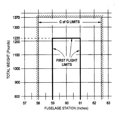
**Note:** For the first flight the total weight and C of G should be within the First flight box shown on the graph.
