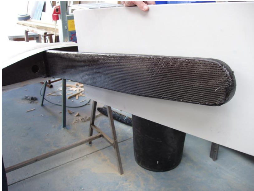
Fig. 11: Port Spar Tang after cloth Lay-up
