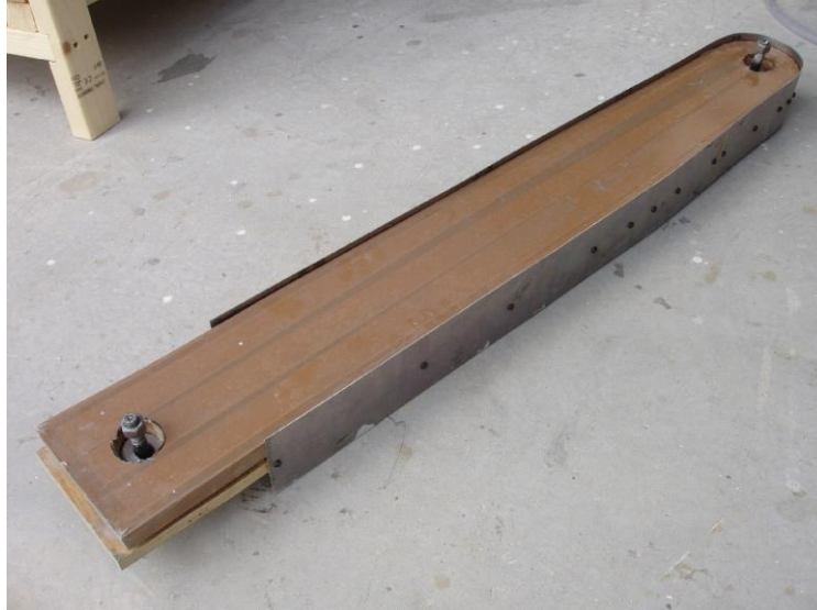
Fig 3: Spar Boom Mould Assembly
