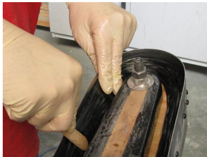
Fig 8: Carbon Rope Lay-up in Progress
