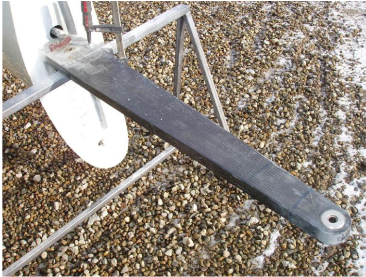
Inspect spar tang on all four surfaces
