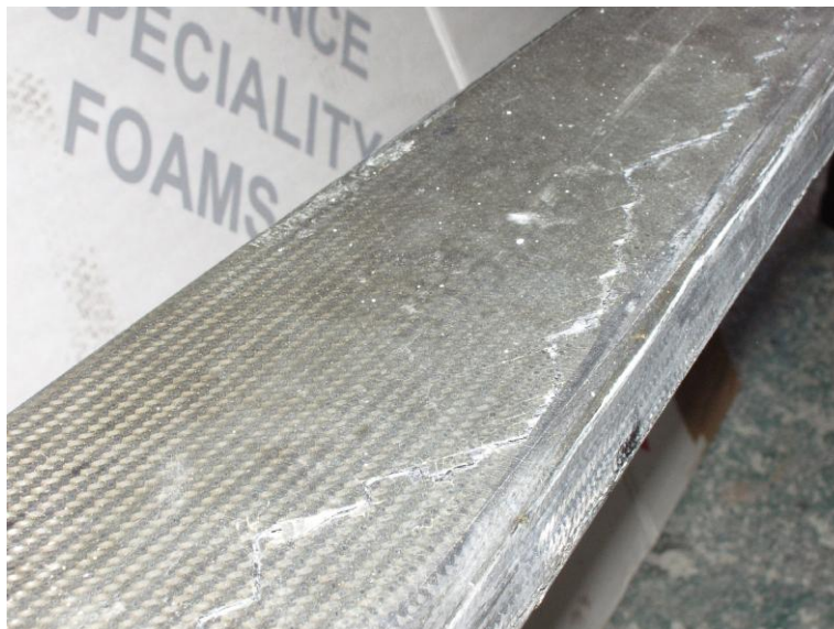
View of cracks that may be present in spar webs
