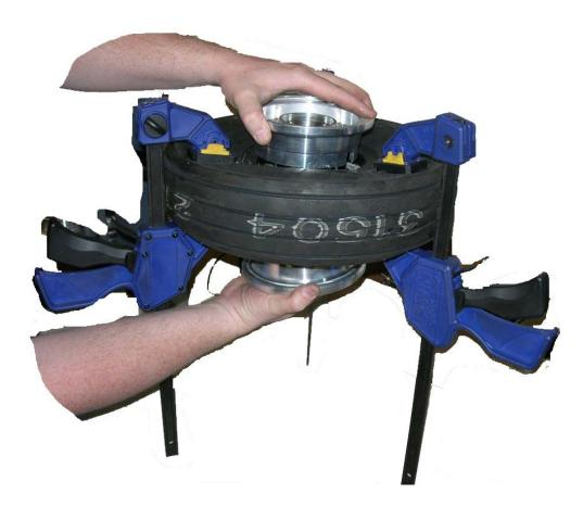
4) WHEEL HALVES MAY NOW BE INSTALLED WITH MATING HALVES ABLE TO TOUCH. TUBE CAN BE INSPECTED CLEAR OF HALVES AND NOT PINCHED. INSERT TIEBOLTS AND SECURE EVENLY. CLAMPS MAY THEN BE RELEASED AND BOLT TORQUED AS REQUIRED.
