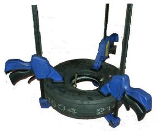
1) USE 3 RACHETING BEAM CLAMPS TO COMPRESS TIRE WITH TUBE INSIDE. COMPRESS BEAD SEATS NARROWER THAN MATING WHEEL HALVES.
