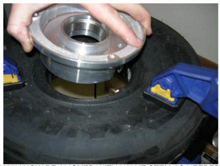
3) WHEEL HALF MAY NOW BE ALIGNED WITH VALVE STEM AS NEEDED
