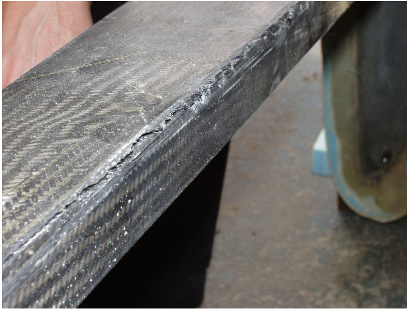
View of cracks that may be present at spar corners
