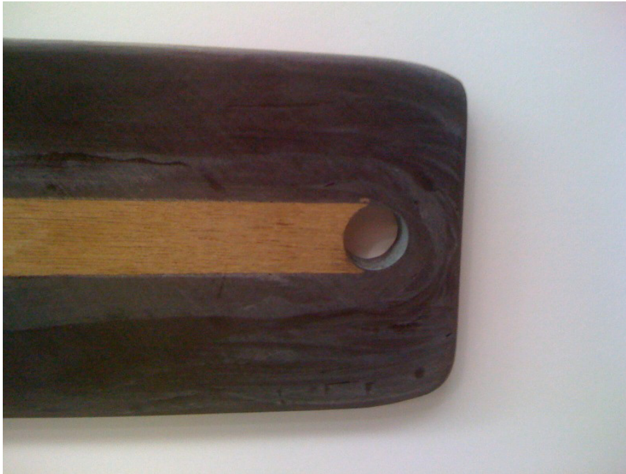
Fig. 10: Truncated Starboard Spar Tang prior to Cloth Lay-up:
