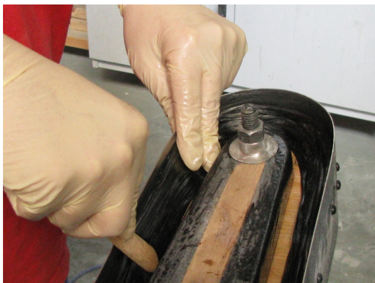
Fig 8: Carbon Rope Lay-up in Progress
